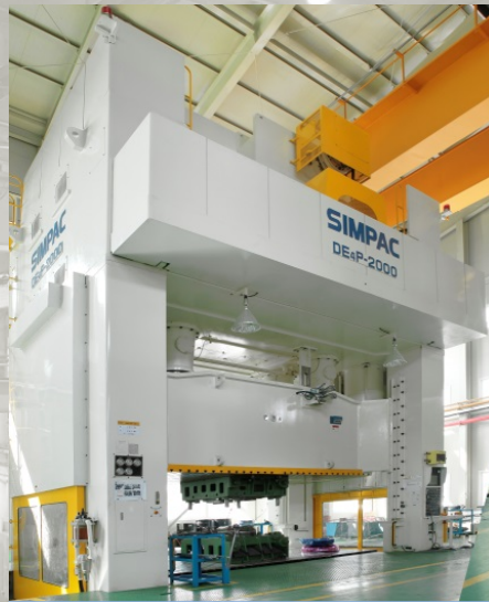
2000T Mechanical Press (5400 X 2500)
